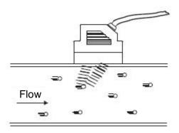
**Step 6:** Press the ON/OFF key. Wait at least 30 seconds before recording a reading. The UFX will automatically turn itself off after 3 minutes.
