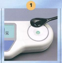
Apply drops of sample into the sensor section until it fills above the indication line.
