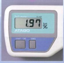
After arrow flashes three times, the display indicates the salinity of the measured sample in percentage.
