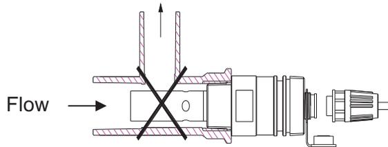
11.3.2 Insufficient water flow: The installation is prone to error measurement due to insufficient water flow.
