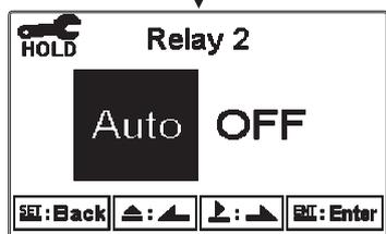
Press or to select for activating REL2 or not. If select OFF, the guide menu goes to setup of clean.
