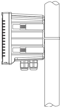
Installation of pipe mounting
