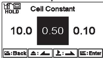
According to the cell constant of the resistivity sensor, press
