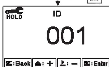
Press or to set the ID number of the transmitter. The valid value is from 1 to 247.
