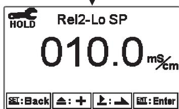
Press or to adjust set-point (SP) value. If the measuring range of conductivity measurement is set as AUTO, then it needs to be set unit( $\mu$ S/cm or mS/cm), value, and decimal point by order.
