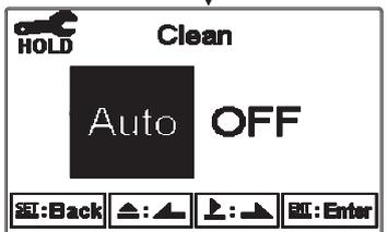
Press or to select for activating Clean or not. If not, the guide menu goes to setup of Analog 1.
