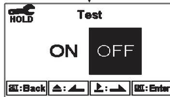
Press or to select for activating a test of Clean or not. If “ON”, the Clean function is in action, and the “WASH” indication light will light up.
