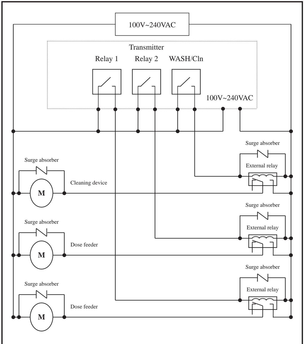
Note: The transmitter built-in miniature relay is necessary to be repaired and replaced by professional technicians. It is recommended to use an external relay (Power Relay) to activate the external equipments.
