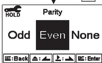
Press or to select Even, or Odd, or None for parity check.
