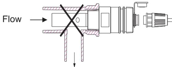
11.3.3 Insufficient immersion: The installation is easy to result in stagnant water inside the cell and thus lead to measurement error.
