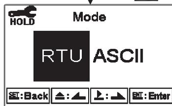
Press or to select RTU or ASCII mode.
