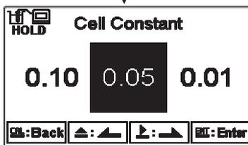
According to the cell constant of the resistivity sensor, press
