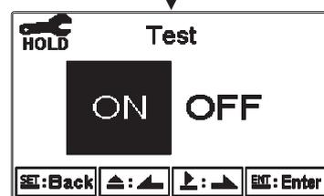
Press or to select for activating a test of REL2 or not. If “ON”, the relay 2 is in action, and the “RELAY2” indication light will light up.
