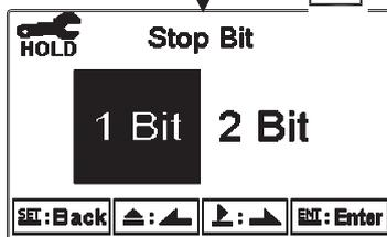
Press or to select stop bit as 1 bit or 2 bit.
