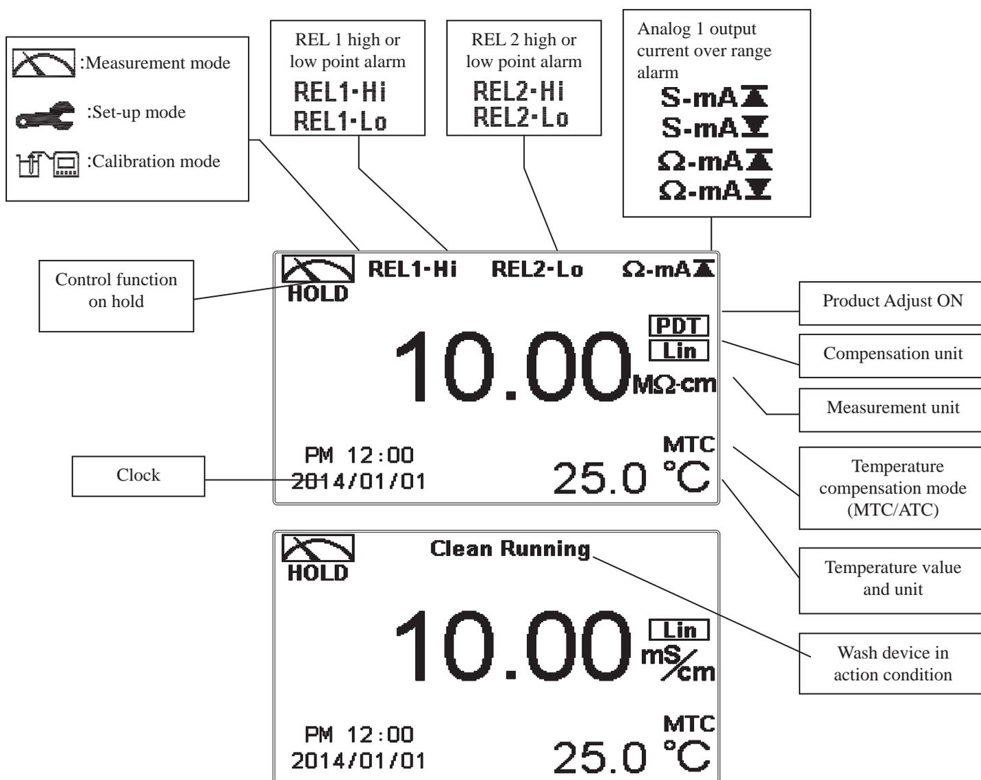
Note: The “HOLD” warning text appears when clean function is activated, or when entering setup menu, or when entering calibration menu. Under HOLD status, the corresponding display and output as follows:
