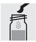
Add 1 level blue microspoon of **CN-3K**, close the cell with the screw cap.
