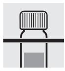
Replace the cell in the rack for complete cooling to room temperature.
