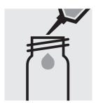
Pipette 10 ml of the sample into a round cell.
