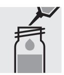
Pipette 4.0 ml of the sample into a reaction cell, close with the screw screw cap, and mix. cap, and mix.
