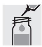
Pipette 1.0 ml of NO<sub>3</sub>-1K into a reaction cell, do not mix.
