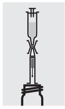
Fill the 10-ml syringe with Add 2 level green 10 ml of reagent AOX-5 and attach the syringe with the column outlet using the connector. Place the top end of the column on an empty cell and rinse the charcoal filling of the column into an empty 16-mm cell.
