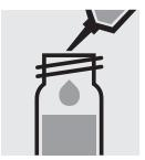
Pipette 6.0 ml of the sample into a reaction cell, close with the screw cap, and mix.
