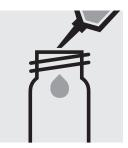
Pipette 5.0 ml of the sample into a reaction cell, close with the screw cap, and dissolve the solid substance.
