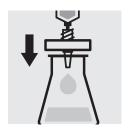
Filter the contents of the syringe into the intended glass vessel.
