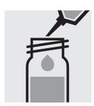
Pipette 0.50 ml of the sample into a reaction cell, **do not mix**.
