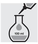
Pipette 5.0 ml of the sample into a 100-ml volumetric flask, fill to the mark with distilled water and mix thoroughly.
