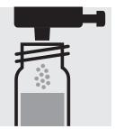
Add 1 dose of  $NH_4$ -1K using the blue dosemetering cap, close the cell with the screw cap.
