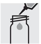
Add 9.0 ml of distilled water (Water for analysis spoon of N-1K. EMSURE®, Cat.No. 116754, is recommended) with pipette.
