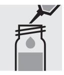
Pipette 1.0 ml of the pretreated sample into a reaction cell, do not
