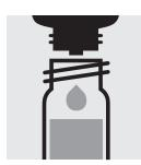
Add 5 drops of Pb-1K into a reaction cell and mix.
