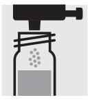
Add 1 dose of **Cr-2K** using the blue dosemetering cap, close the reaction cell with the screw cap.
