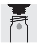
Add 6 drops of **Cr-3K** into a reaction cell, close with the screw cap.
