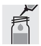
Pipette 0.50 ml of Na-1K Add 0.50 ml of the into a reaction cell and mix.
