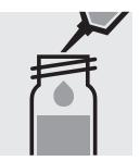
Add 1.0 ml of NO<sub>3</sub>-1K with pipette, close the cell with the screw cap, and mix. Caution, cell becomes hot!
