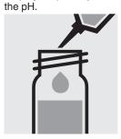
Add 7.0 ml of distilled water with pipette to the second reaction cell, close with the screw cap, and mix. (Blank)
