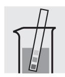
Check the pH of the sample, specified range: pH 2- 12.
