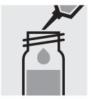
Add 0.50 ml of reagent 2 with pipette, close the cell with the screw cap, and mix.
