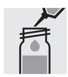
Pipette 1.0 ml of the sample into a reaction cell, **do not mix**.
