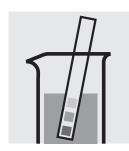
Check the pH of the sample, specified range: pH < 3. If required, add dilute sulfuric acid drop by drop to adjust the pH.
