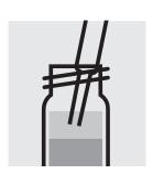
Aspirate the clear upper phase from the tube with pipette.
