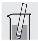
Check the pH of the sample, specified range: pH 3 - 8. If required, add dilute sodium hydroxide solution or sulfuric acid drop by drop to adjust the pH.
