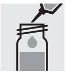
Add 5.0 ml of **sulfuric acid 40%**, close the cell with the screw cap, and mix.
