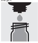
Add 5 drops of  $O_2$ -2K, close the cell with the screw cap, and shake for 10 seconds.
