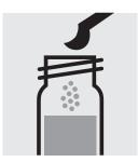
Add 1 level green microspoon of **Cd-2K**, close the cell with the screw cap.
