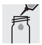
Pipette 5.0 ml of the sample into an empty round cell (Empty cells, Cat.No. 114724).
