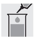
Pipette 0.20 ml each of CI-1 into two test tubes.
