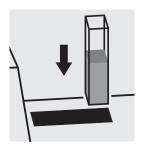
Place the cell into the cell compartment.
