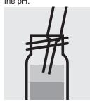
Aspirate the organicclear upper phase from the tube with pipette and dry over sodium sulfate anhydrous (Cat.No. 106649).
