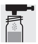
Add 1 dose of **CN-1** using the green dosemetering cap, close the cell with the screw cap.
