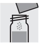
Add 1 powder pack of **Oxyscav 1** and close with the screw cap.
