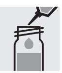
Pipette 5.0 ml of the sample into a reaction cell, close with the screw screw cap, and mix. cap, and mix.
