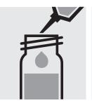
Add 2.0 ml of the sample with pipette, close the cell with the screw cap, and mix.
