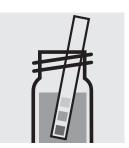
Check the pH of the sample, specified value: pH 6.5. If required, add dilute sodium hydroxide solution or sulfuric acid drop by drop to adjust the pH.
