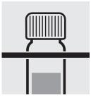
Remove the cell from the thermoreactor and place in a test-tube rack to cool to room temperature: pretreated sam-
