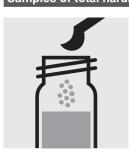
Add 1 level grey microspoon of Pb-2K to the already measured cell, close the cell with the screw cap.
