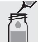
Carefully pipette 5.0 ml of the depleted blank tightly with the screw cap, cell, close tightly with the screw cap, and mix vigorously. Caution, the cell
