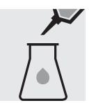
Place 350 ml of the sample into an Erlenmeyer flask with ground joint.
