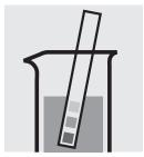
Check the pH, specified range: pH 2.0 – 2.5. If required, add dilute sodium hydroxide solution or sulfuric acid drop by drop to adjust the pH.
