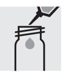
Pipette 10 ml of the sample into an empty round cell (Empty cells, Cat.No. 114724).
