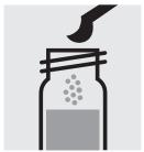
Add 1 level blue microspoon of **F-1K** to each cell, close with the screw cap.
