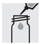
Pipette 5.0 ml of the sample into a round cell.
