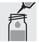
Add 4.0 ml of the sample with pipette into a reaction cell, close the cell with the screw cap.
