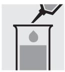
Add 0.50 ml of PO<sub>4</sub>-1 with pipette and mix.
