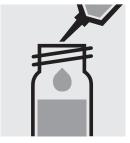
Pipette 10 ml of distilled water into a second reaction cell, close with the screw cap, and mix. (Blank)
