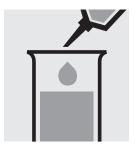
Pipette 5.0 ml of distilled Add to each tube 1.0 ml water (Water for analysis of F-1 with pipette and EMSURE®, Cat.No. 116754) into a second test tube. (Blank)
