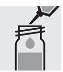
Pipette 5.0 ml of the sample into a reaction cell, **do not mix!**
