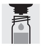
Add 6 drops of K-1K, close the cell with the screw cap, and mix.
