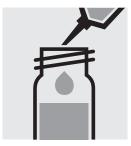
Add 1.0 ml of **OA-3** with pipette, close the cell with the screw cap, and mix
