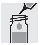
Add 1.0 ml of **B-1** with pipette, close with the screw cap, and mix.
