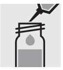
Add 0.50 ml of the sample with pipette, close with the screw cap, and
