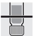
Remove the cell from the thermoreactor and let it, **standing on its head**, to cool for 1 hour.
