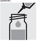
Add to each vessel 0.50 ml of **Si-3** with pipette, close with the screw cap, and mix.
