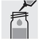
Pipette 10 ml of the sample into a reaction cell, close with the screw cap, and mix.
