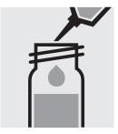
Add 0.50 ml of the sample with pipette, close with the screw cap, and mix.
