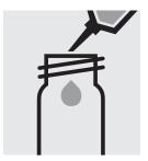
Pipette 5.0 ml of the 1:500 dilute sample into an empty round cell (Empty cells, Cat. No. 114724).
