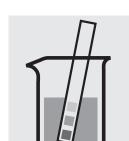
Check the pH of the sample, specified range: pH 4- 10. If required, add dilute sodium hydroxide solution or hydrochloric acid drop by drop to adjust the pH.
