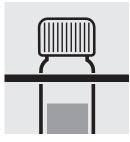
Remove the cell from the thermoreactor and place in a test-tube rack to cool to room temperature: **pretreated sample**.
