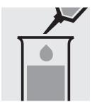
Pipette 5.0 ml of the sample into a test tube.
