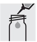
Add 10 ml of the sample into an empty round cell (Empty cells, Cat.No. 114724).
