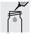
Pipette 5.0 ml of the **pretreated sample** into a reaction cell, close with the screw cap, and dissolve the solid substance.
