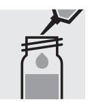
Pipette 1.0 ml of the sample into a reaction cell, close with the screw cap, and mix.
