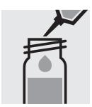
Pipette 7.0 ml of the sample into a reaction cell, close with the screw cap, and mix.
