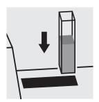
Place the cell into the cell compartment.
