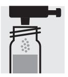
Add 1 dose of P-3K using the blue dosemetering cap, close the cell with the screw cap.
