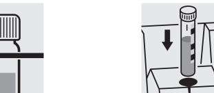
Configure the photometer for blank-measurement.
