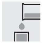
Transfer the solution into a 50-mm cell.
