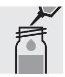
Add 1.0 ml of N-3K with pipette, close the cell with the screw cap, and mix. Caution, cell becomes hot!
