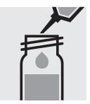
Pipette 0.50 ml of **CI-1K** into a reaction cell, close with the screw cap, and mix.
