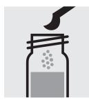
Add 1 level grey microspoon each of SO<sub>3</sub>-1K into two reaction cells, close with the screw cap.
