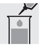
Add to the second tube 10 ml of of distilled water (Water for analysis ÈMSURE®, Cat.No. 116754, is recommended) with pipette and mix. (Blank cell)
