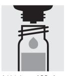
Add 4 drops of **SO**<sub>4</sub>**-4** to the filtrate, close the test tube with the screw cap, and mix.
