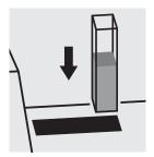
Place the cell into the cell compartment.
