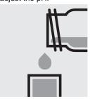
Transfer the solution (when possible without sediment) into a corresponding rectangular cell.
