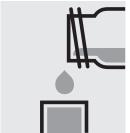
Transfer the solution into a corresponding rectangular cell.
