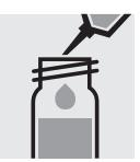
Add 5.0 ml of NO<sub>3</sub>-2 with pipette into the cell. Close the cell with the screw cap.
