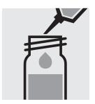
**Immediately** add 1.5 ml of **NO**<sub>3</sub>**-2** with pipette.
