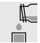
Transfer the solution into a rectangular cell.
