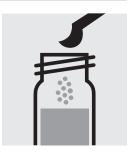
Add 1 level grey microspoon of SO<sub>3</sub>-1K into a reaction cell, close with the screw cap.
