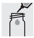
Pipette 5.0 ml of NO₃-1 into a dry empty round cell (Empty cells, Cat. No. 114724).
