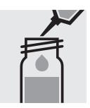
Add 6.0 ml of **B-6** with pipette, close with the screw cap, and mix.
