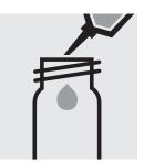
Add 9.0 ml of distilled water (Water for analysis spoon of N-1K. EMSURE®, Cat.No. 116754, is recommended) with pipette.
