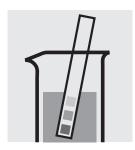
Check the pH of the sample, specified range: pH 4-9. If required, add dilute sodium hydroxide solution or sulfuric acid drop by drop to adjust
