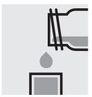
Transfer the solution into a rectangular cell.
