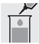
Pipette 5.0 ml of distilled water (Water for analysis EMSURE®, Cat.No. 116754, is recommended) into a test tube.
