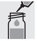
Add 5.0 ml Isobutyl-methylketone GR (Cat.No. 106146) with pipette, close the cell with the screw cap.
