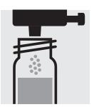
Add 1 dose of **F-1K** using the blue dosemetering cap, close the cell with the screw cap.
