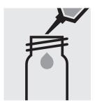
Pipette 10 ml of the sample into into an empty round cell (Empty cells, Cat.No. 114724).
