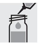
Add 1.0 ml of NO<sub>3</sub>-1K with pipette, close the cell with the screw cap, and mix. Caution, cell becomes hot!
