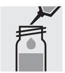
Pipette 1.0 ml of the sample into a reaction cell, close with the screw screw cap, and mix. cap, and mix.
