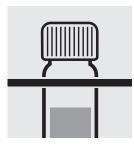
Replace the cell in the rack for complete cooling to room temperature. Very important!
