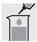
Pipette 10 ml of sample into a glass vessel.
