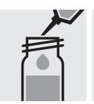
Pipette 2.0 ml of the sample into a reaction cell, close with the screw cap, and mix.
