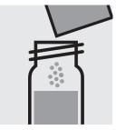
Add 1 powder pack of **Molybdenum HR3** and close with the screw cap.
