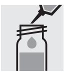
Pipette 4.0 ml of the sample into a reaction cell. Close with the screw cap.
