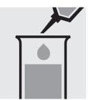
Pipette 8.0 ml of distilled Add 0.50 ml of the water (Water for analysis sample with pipette and EMSURE®, Cat.No. 116754, is recommended) into a test tube.
