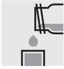
Transfer the blank into a rectangular cell and measure **immediately**.
