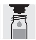
Add 15 drops of **B-5**, close with the screw cap, and mix.
