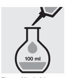
Pipette 25 ml of the sample into a 100-ml volumetric flask, fill to the mark with distilled water and mix thoroughly.
