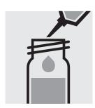
Pipette 2.0 ml of the sample into a reaction cell, **do not mix**.
