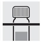
Remove both cells from the thermoreactor and place in a test-tube rack to cool.
