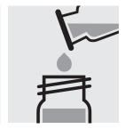
Fill the solution into a round cell.
