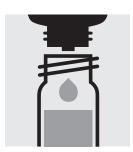
Add 2 drops of **Ni-2K**, close the cell with the screw cap, and mix.
