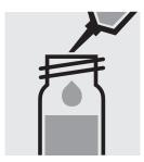
Carefully pipette 2.0 ml of the sample into a reaction cell, close tightly with the screw cap, and mix vigorously.
