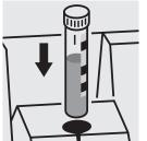
Place the blank cell into the cell compartment. Align the mark on the cell with that on the photometer.
