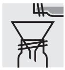
Filter the content of the test tube with a round filter into another test tube with screw cap.
