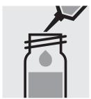
Add 7.0 ml of the sample with pipette to one reaction cell, close with the screw cap, and mix.
