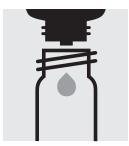
Place 6 drops of Cl<sub>2</sub>-1 into a round cell.
