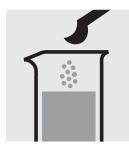
Add 1 level green microspoon of **Zn-1K** and shake to dissolve the solid substance: **sample-reagent mixture**.
