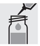
Add 5.0 ml of **sulfuric acid 40%**, close the cell with the screw cap, and mix.
