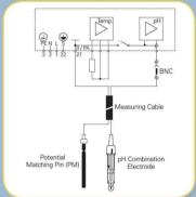
Symmetrical mode avoids grounding the reference electrode by reconfiguring the input to a floating differential mode. The electrical noise appears equally on the pH and reference electrodes, and is therefore rejected by the operational amplifier.
