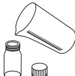
Fill a clean and dry vial up to the mark with dilution water (see chapter 2.3.7.1 Preparing Dilution Water).
