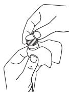
Take care to handle the vial by the top. Wipe the vial with the supplied cleaning tissue to remove waterdrops and finger prints.
