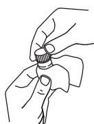
Hold the vial by the cap and clean it with the supplied cleaning tissue to remove water spots and finger prints.
