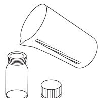
Fill a clean and dry vial with the water sample up to the mark (approx. 12 ml).
