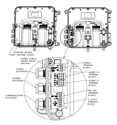
**Figure 1: Electrical Connections for the Instrument**
