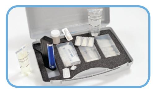
The test uses a pre-dispensed dry blended reagent formulation for total *coliform* and *E.coli*. Positive samples are detected by a visible colour change. Performing the *coliform* test is simple. Add one sachet to 100ml of water, incubate and note the colour change. The formation of a yellow colour in 24 hours or less indicates the presence of total *coliforms*. Positive tubes are then checked for the presence of *E.coli* by looking for fluorescence under UV light.
