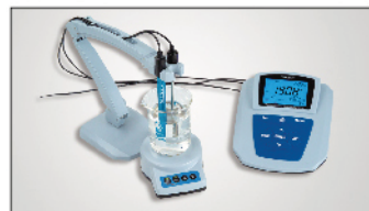
MP518 Calcium Ion Concentration Meter
