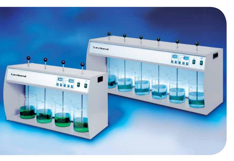
Floc testers with continuously variable stirring speed for laboratory and field use
