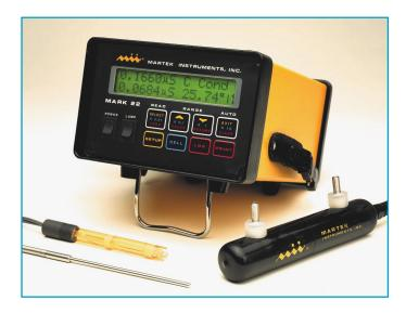
While Martek Instruments offers its own certified, unbreakable conductivity reference cells and pH sensor, the Mark 22 can also be used with any conductivity reference cell or pH electrode regardless of manufacturer.
