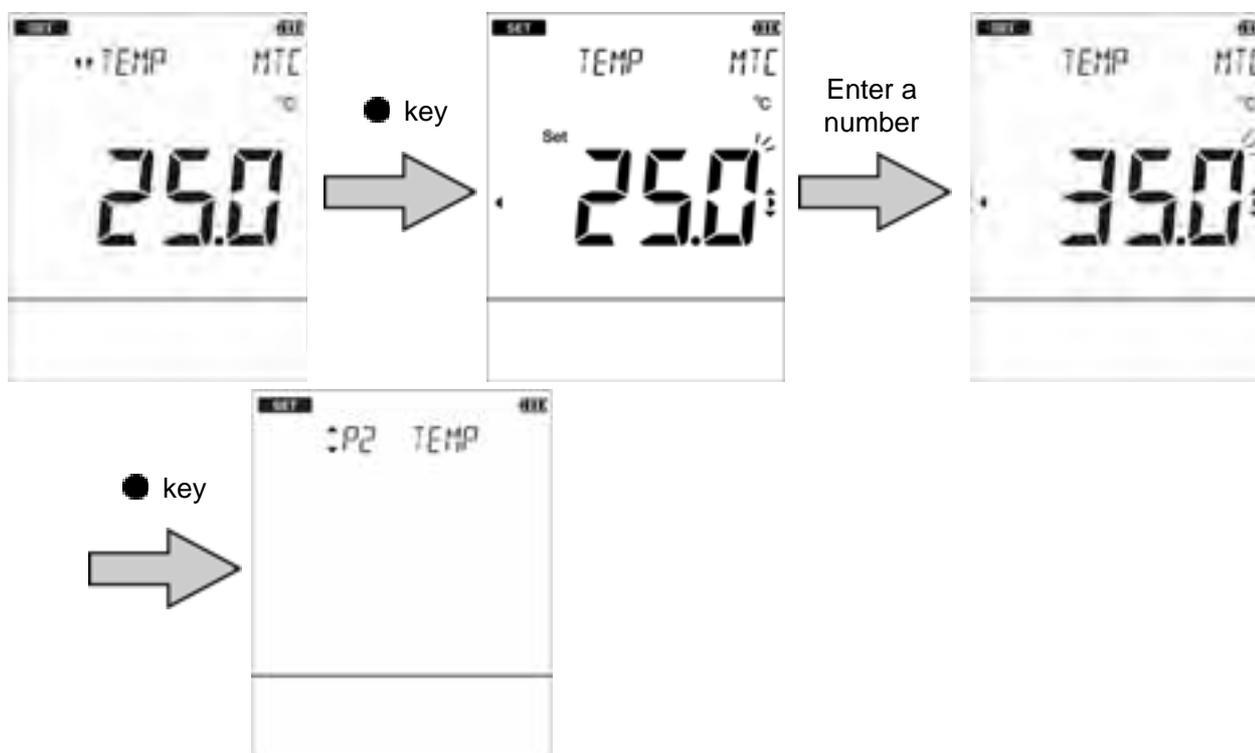
To return to the measurement mode, press the
