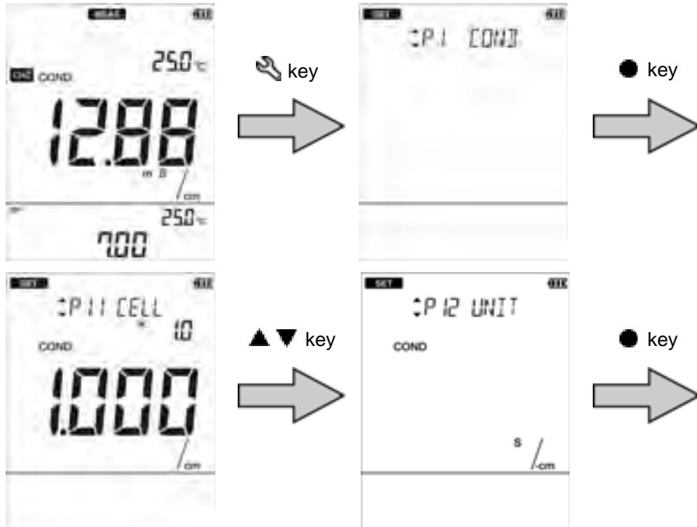
4. Press the ◀▶ key to select the unit and press the ● key to confirm selection.
