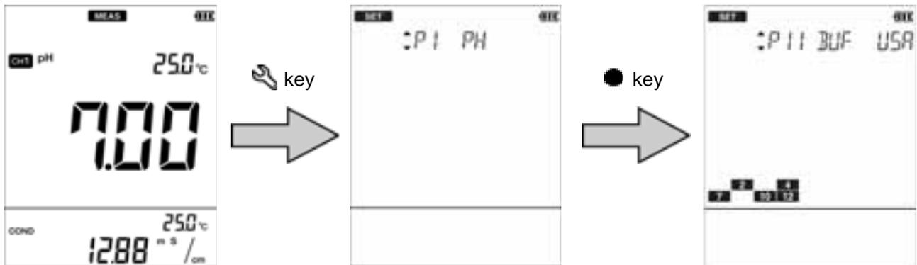
4. Press the ◀▶ keys to select "USA", "NIST", or "CUST" according to the standard solution to be used and then press the ● key to confirm selection.
