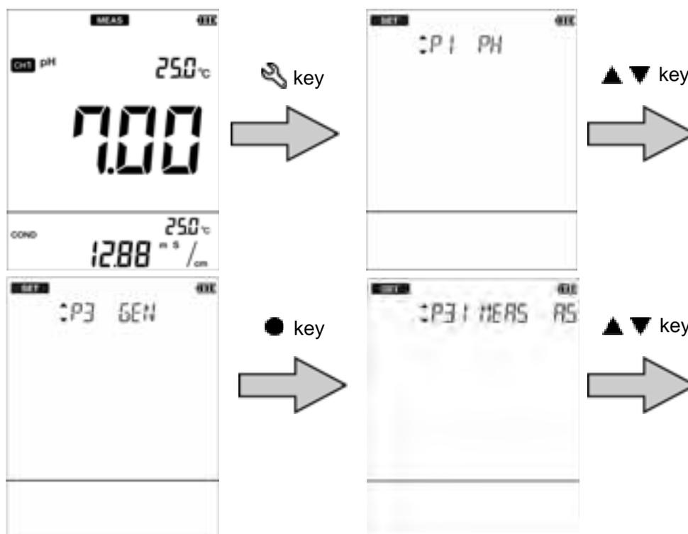
3. Press the ▲▼ keys to select "DATE" (date and time setting) and then press the ● key.
