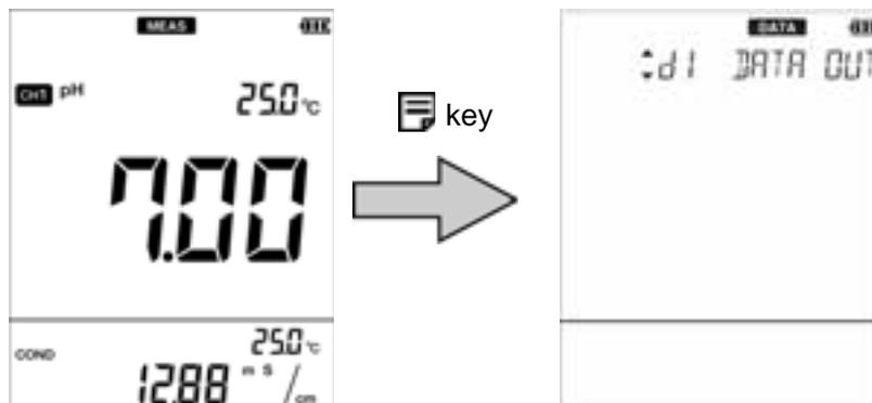
2. Press the ▲▼ keys to select "DATA CLR" (delete saved data) and then press the ● key to confirm.
