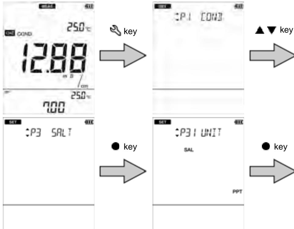
4. Press the ◀▶ keys to select the unit and then press the ● key to confirm selection.
