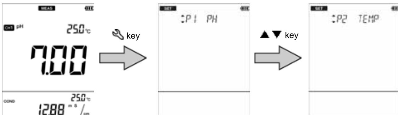
5. Make sure that "ATC" is displayed, and press the
