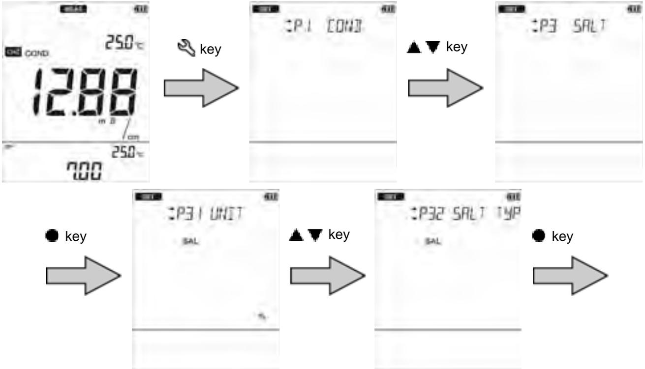
4. Press the ◀▶ keys to select the salinity calculation method and then press the ● key to confirm.
