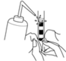
3. Immerse the conductivity cell in the sample solution.
