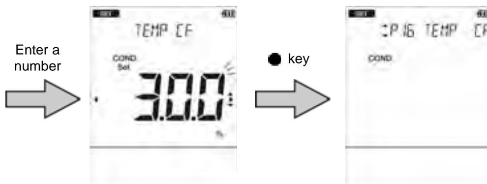
To return to the measurement mode, press the
