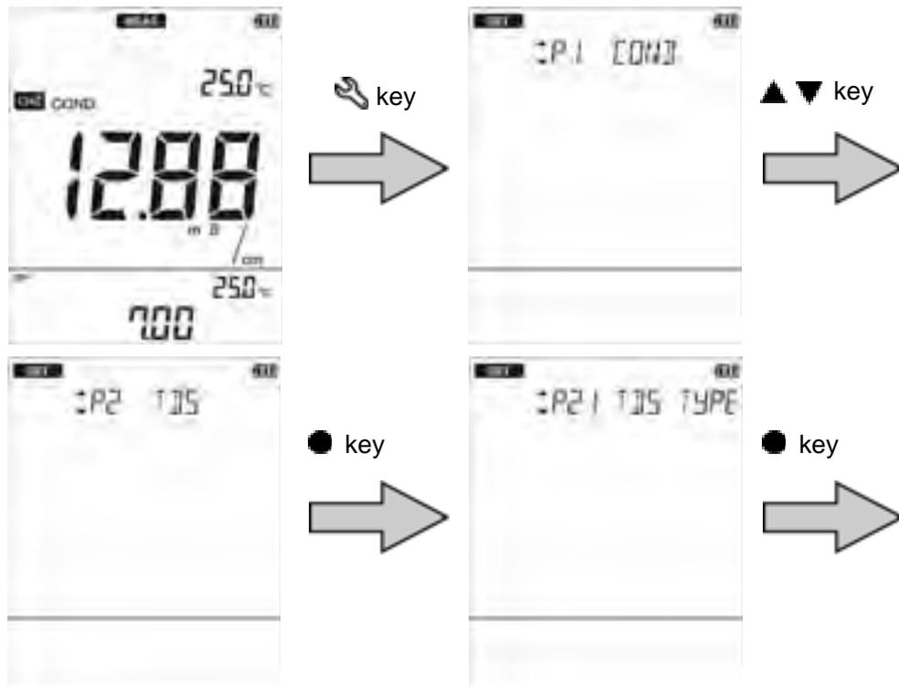
4. Press the ◀▶ keys to select the TDS method and then press the ● key.
