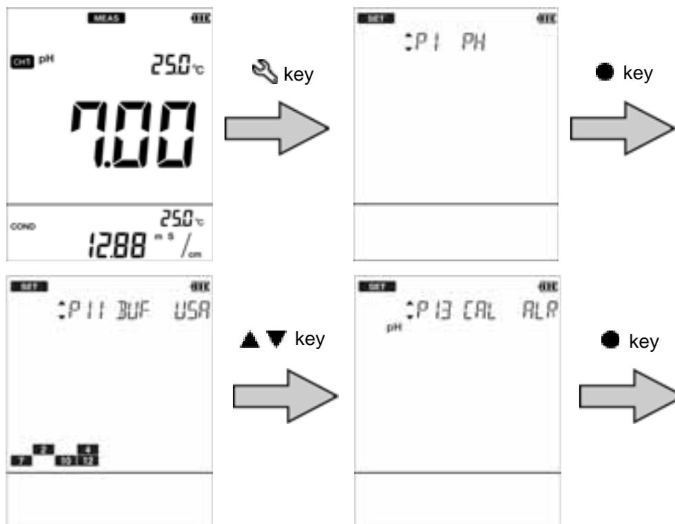
4. Enter the setting period of the calibration interval alarm and then press the
