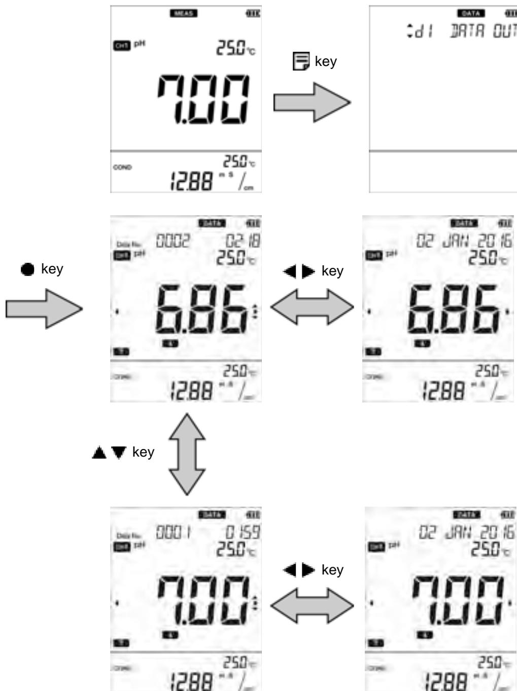
To return to the measurement mode, press the
