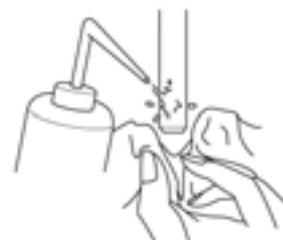
2. **Open the internal solution filler port of the electrode.**
