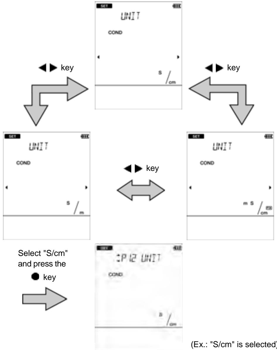
To return to the measurement mode, press the 🏠 key.
