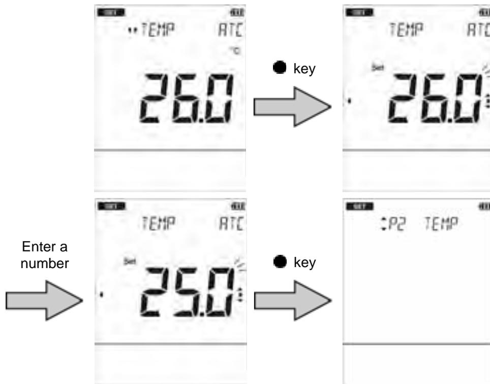
To return to the measurement mode, press the
