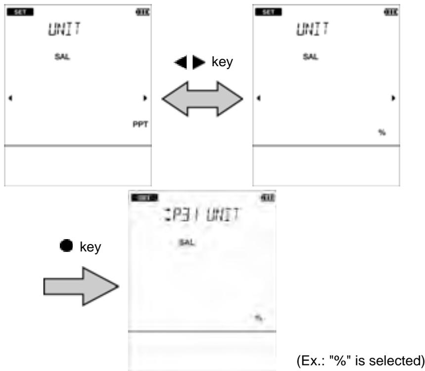
To return to the measurement mode, press the ⏪ key.
