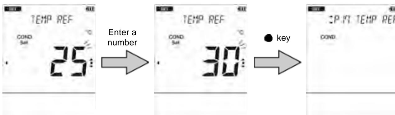
To return to the measurement mode, press the
