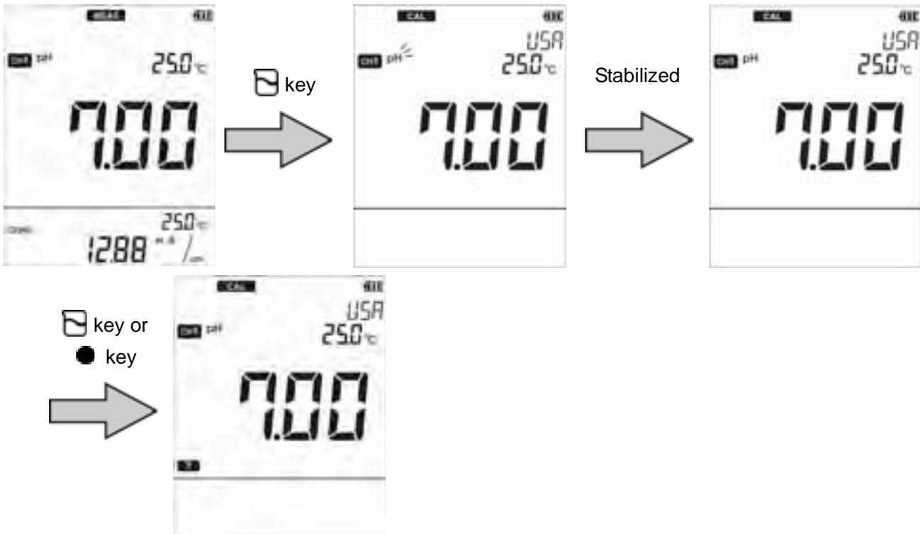
6. Perform the 2nd point calibration. As with the step 1., clean the pH electrode and immerse it in the pH 4 standard solution. As with the step 3., immerse at least 3 cm from the tip of the pH electrode.
