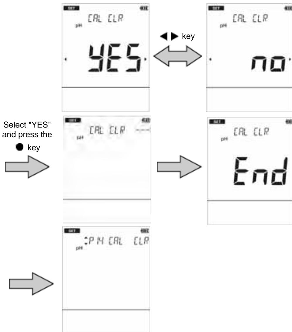
To return to the measurement mode, press the
