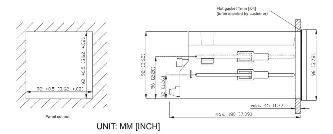
Transmitter housing for panel mounting: protection class IP 54 (front), IP 40 (housing)
