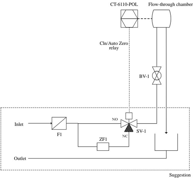
(B) Auto-Zero calibration piping configuration
