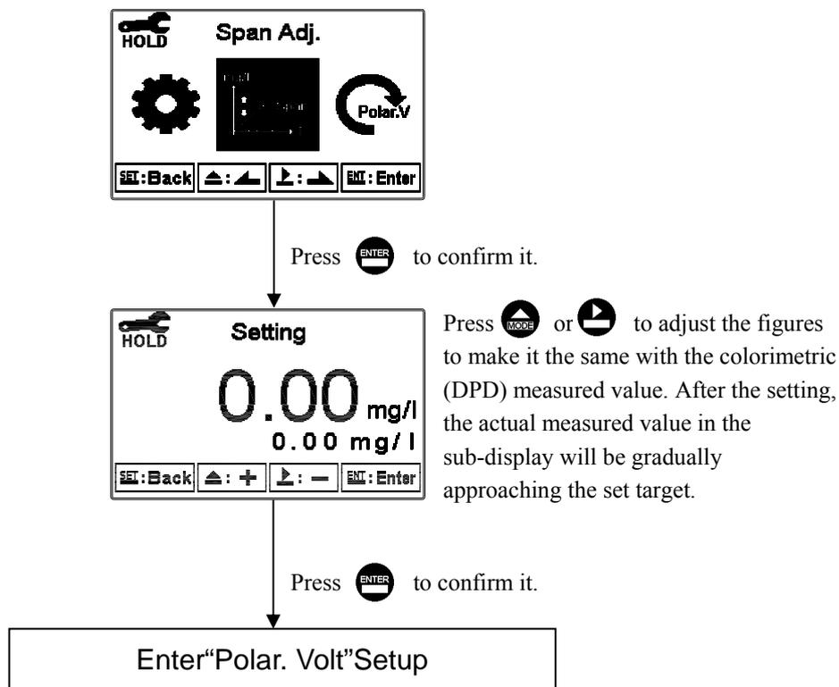
**Note:** After the span adjustment, the "Overview of Setting" display will show the input value of span setting and the relative drifting (span adj.) of the last span calibration. It may help for electrode aging determination. See following illustration for an example.
