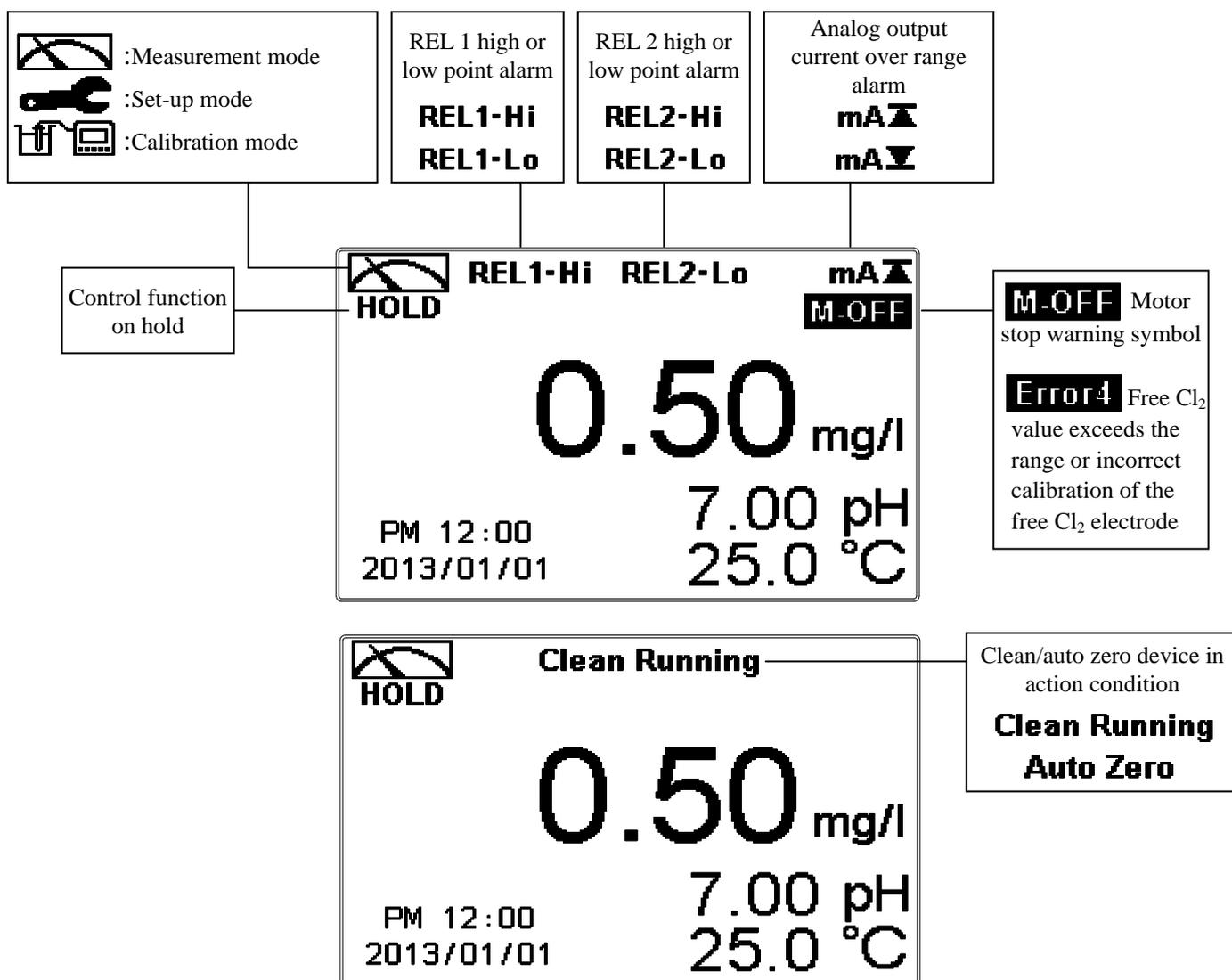
Note: The “HOLD” warning text appears when clean/auto zero function is activated, or when entering setup menu, or when entering calibration menu. Under HOLD status, the corresponding display and output as follows:
