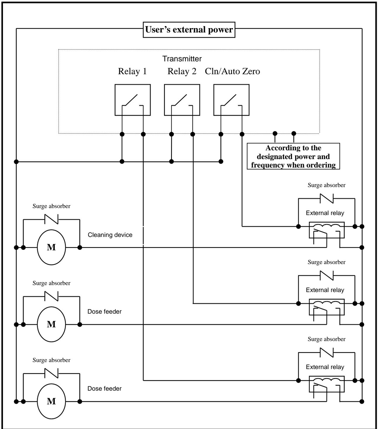
Note: The transmitter built-in miniature relays is necessary to be repaired and replaced by professional technicians. It is recommended to use an external relay (Power Relay) to activate the external equipments.
