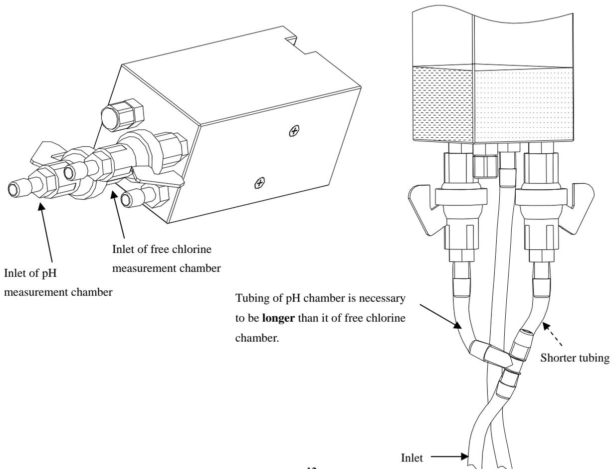
**2.3.3 External piping configuration** (Just for reference, not included in the standard & optional accessories list, users may select for installation according to the field conditions.)
