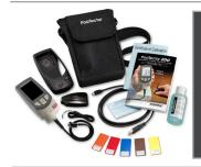
**Comes complete** with PosiTector gage body, 200D probe, couplant (ultrasonic gel), precision plastic shims, protective rubber holster with belt clip, wrist strap, 3 AAA alkaline batteries, instructions, protective lens shield, convenient carrying case, Long Form Certificate of Calibration traceable to NIST or PTB, USB cable, PosiSoft Software, two (2) year warranty.
