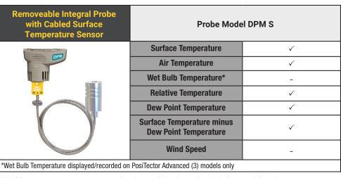
DPM S Probe measures and records climatic conditions including: Relative humidity, air temperature, surface temperature, dew point temperature and difference between surface and dew point temperatures. Includes the ambient temperature and humidity sensors from PosiTector DPM Integral Probe plus a magnetic surface temperature sensor with armored cable (also accepts other optional K-type sensors).
