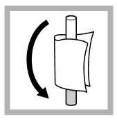
**10.** Invert the vial assembly so the indicator vial is on the bottom. Clean the indicator vial.
