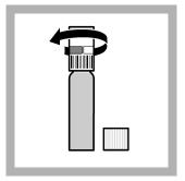
4. When the shake time is complete, remove the cap from a blue indicator vial. Immediately install and tighten a double cap on the indicator vial with the barcode label toward the vial.
