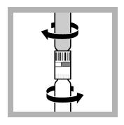
**9.** Tighten the double cap on both vials.
