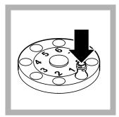
2. Insert the uncapped sample vial into the TOC-X5 shaker. Make sure that the vial is pushed all the way down into the shaker. Move the fan over the vial.
