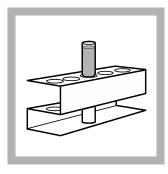
8. Let the vial assembly cool completely to room temperature. Make sure that the vials cool completely. Warm vials will give high results.
