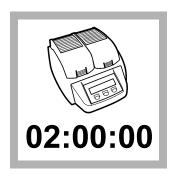
7. Increase the vial assembly temperature for 2 hours at 100 °C.
