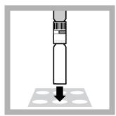
**6.** Insert the vial assembly into the DRB reactor (indicator vial on top).
