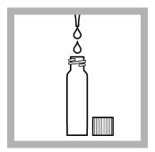
1. Remove the cap from a clear vial. Use a pipet to add 2 mL of sample to the vial.
