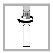
**5.** Immediately invert the indicator vial, then install and tighten the other side of the double cap on the sample vial. Hold the vial assembly vertically.
