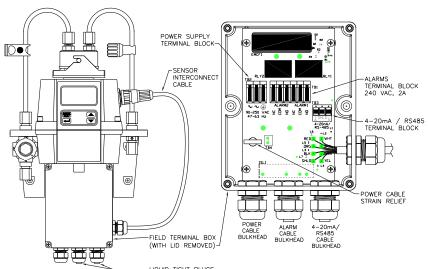
Figure 5: Electrical Connections for the Instrument
