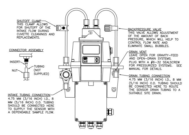
**Figure 4: Recommended Plumbing for the Instrument**
