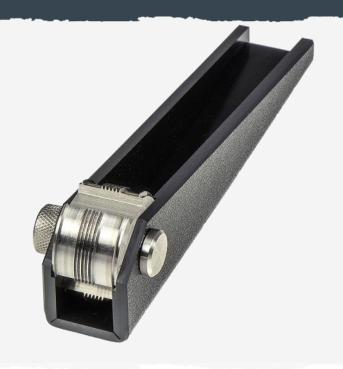
Repeat this operation making further parallel cuts, crossing the original cuts at 90° so that a lattice pattern is formed.
