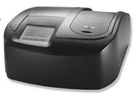
The Hach DR 5000 UV-Vis Laboratory Spectrophotometer offers a broad range of water analysis methods with more than 240 pre-programmed tests. Automatic method detection capability with TNTplus reagents reduces test time and potential errors. The intuitive touch screen interface makes this instrument easy to use.
