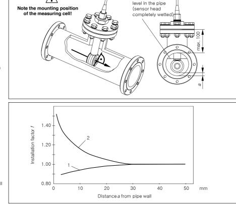
Installation factor f in dependence on distancea from pipe wall
