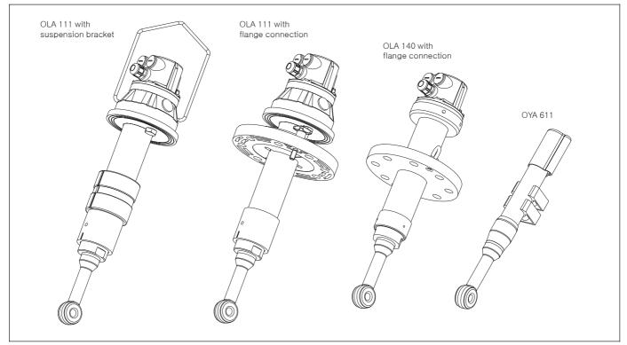
Assembly mounting of measuring cell, G 3 version
