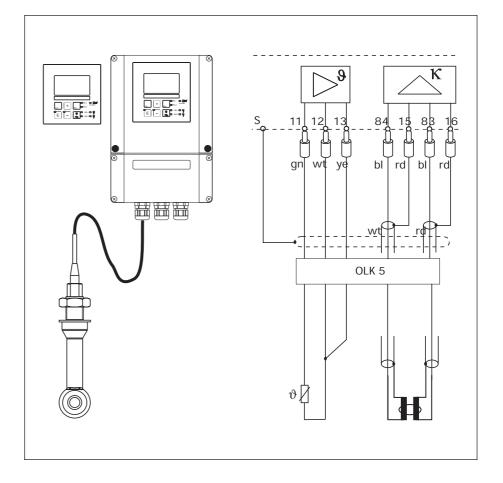
Cable connection at transmitter OLM 223/253
