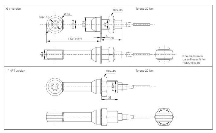
Dimensions: Versions with G ≩ thread (top) and 1" NPT thread (bottom)
