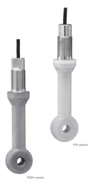
The conductivity sensor OLS 50 is specially suitable for use in the chemical industry and in process engineering. The six-decade measuring range and high chemical resistance of the material in contact with the medium (PFA or PEEK) permit this sensor to be used in virtually any application conceivable. The whide temperature range of -20 to +125 °C (+18 0 °C) leaves nothing to be desired.
