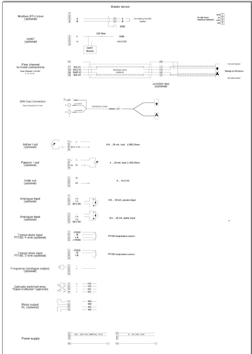
Drawing 3: Electrical connection diagram for the KATflow 150 flowmeter
