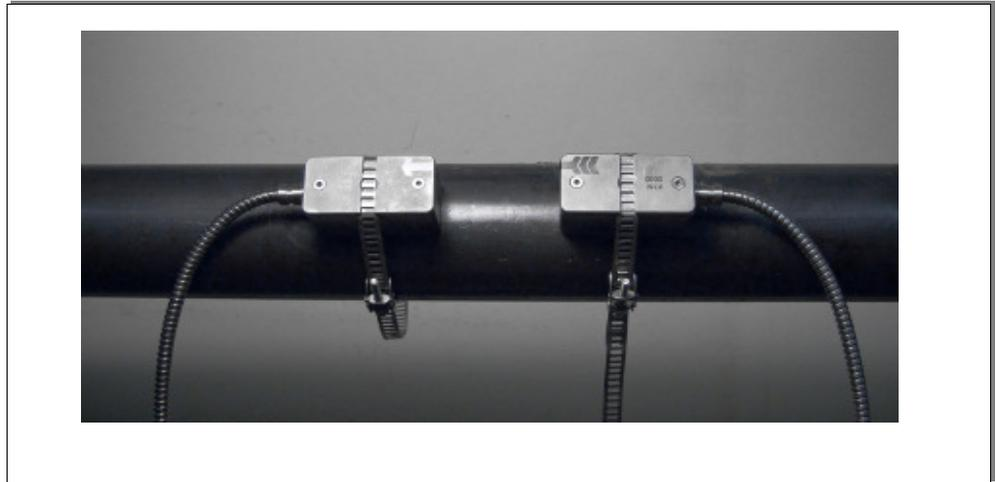
*Illustration 8: Sensor mounting with tension straps and clamps*
