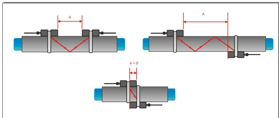
Illustration 3: Clamp-on sensor mounting configurations and sensor spacing
