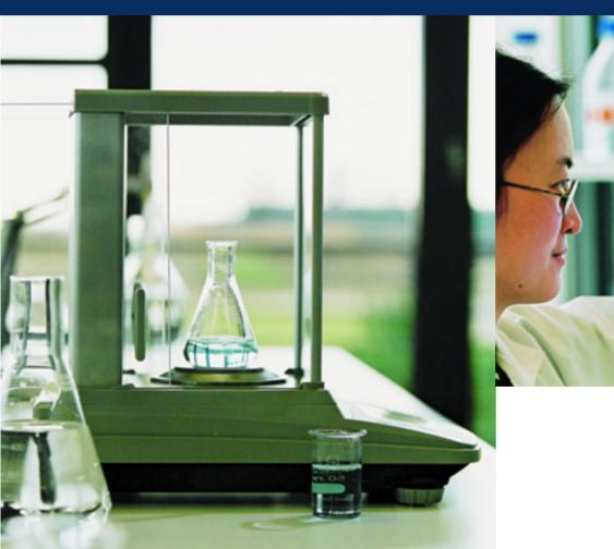
Additional features: integrated overload protection, stable placement on oversized feet, a leveling bubble, a durable, sealed keypad to protect electronic components, and a weigh-below port.
