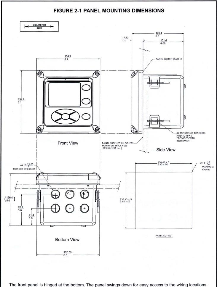
The front panel is hinged at the bottom. The panel swings down for easy access to the wiring locations Panel mounting seal integrity (4/4X) for outdoor applications is the responsibility of the end user.
