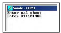
YSI recommends that your replace your sensor membrane after 1 year of use by purchasing the 6155 Optical DO Membrane Replacement Kit. This kit will be supplied with a new set of coded constants which characterize the new membrane and they MUST be entered via the Calibrate|Optic X – Dissolved Oxy|Enter Cal Sheet selection as show above. Once the new constants have been entered in coded form they will be transferred to the probe and will be visible in uncoded form in Advanced|Cal Constants.
