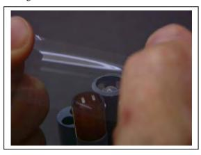
Hold the membrane so that all four corners are supported, but do not stretch the membrane laterally.
