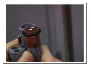
Install a new O-ring by placing one side of the O-ring in the groove and rolling into place across the membrane and into the groove on the opposite side of the probe face. Avoid touching the probe face with
