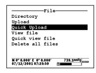
After the sonde file has been uploaded to the 650, the data is resident in the flash memory of both sonde and 650. Note that, if you choose to upload files from the sonde in CDF or ASCII format, the files will be characterized by a .txt extension in the 650 Directory and will NOT be viewable on the 650 display. To view the files, you must first transfer them from the 650 to your PC and then open them in a spreadsheet.
