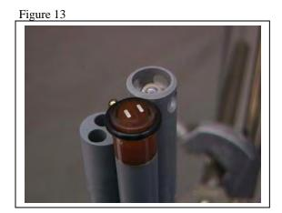
If the installation has been done properly, the finished product should have no bubbles, wrinkles, or tears as shown in Figure 13 above.
