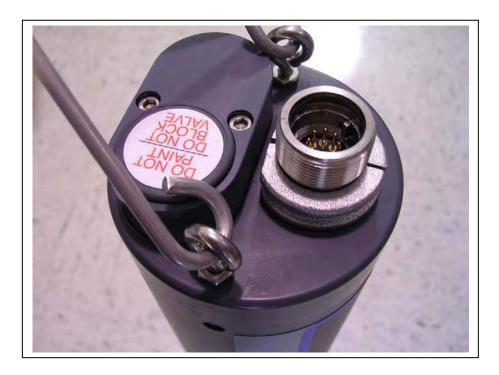
For the 6600-style sondes, first remove the pressure-relief battery lid and set it aside for later installation. The position the zinc anode onto the sonde connector as shown in Figure 4 above, leaving a small gap between the bottom of the anode and the top of the sonde. Make sure that the flat sides of the anode parts are next to the battery lid as shown.
