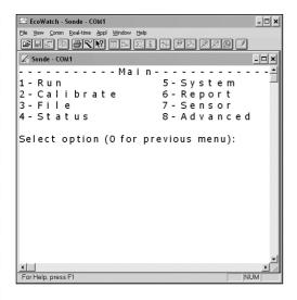
6. After establishing connection with EcoWatch, you can configure sonde settings including date/time, sensors, logging, setup, and access stored files.
