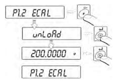
Balance will display a command ordering unloading of weighing pan unloAd (weighing pan should be empty). When weighing pan is unloaded, press PRINT key. The balance determines mass of empty pan. Place an external adjustment weight with mass determined on balance's display and press PRINT key. On completing adjustment process the balance returns to submenuP1.2 ECAL.
