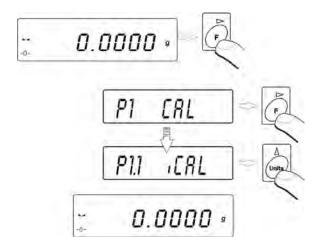
The balance automatically enters internal adjustment mode. During adjustment process do not load the weighing pan with any load. On completion of adjustment process, balance saves its result in memory and returns to weighing mode.
