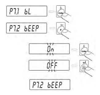
OFF – signal of pressing function key disabled On – signal of pressing function key enabled.
