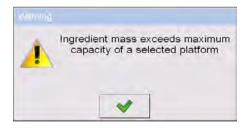
3) – in case of declaring the value of the low deviation as greater than the declared ingredient mass, the software displays the following message:
