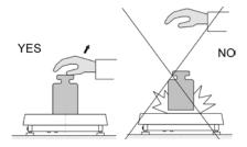
Loads should be placed in the centre of the pan (eccentric errors are outlined in PN-EN 45501 chapter 3.5 and 3.6.2):
