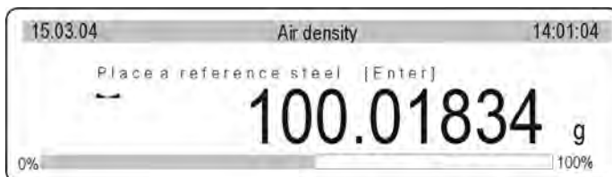
Fig. 28-9. Air buoyancy correction – determining mass of a stainless steel mass standard
