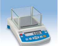
PS/X series of precision balances feature large graphic backlit display and extended user menu. The balances comprise all the features and functions of balances series X and also the newest electronic and mechanical solutions and upgraded software.
