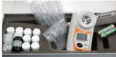
The kit comes complete with 10 bottles of quinone reagent solutions (5ml each), a micropipette, 10 micropipette tips, 10 disposable plastic pipettes, 1 bottle of calibration solution, and 2 AAA batteries.
