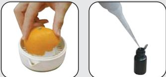
Pipette 0.1ml (100μl) of the sample and dispense it into the quinone reagent solution.
