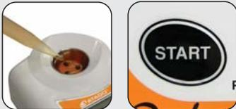
Fill the sample stage with the solution, and then press the START key.
