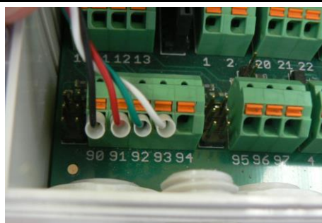
Detailed view of the terminal box: connection area for digital sensors
