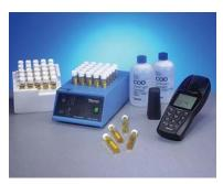
COD Reactor, Test Reagents and Standards with AO4000 Meter
