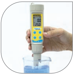
Step 1: Immerse tester sensor in solution
