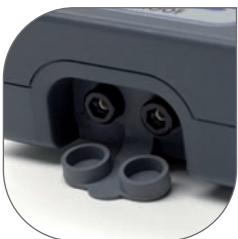
Waterproof external power input
