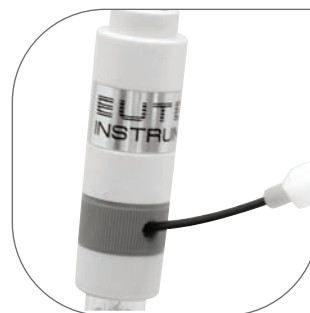
Pour in reference electrolyte with the refilling bottle
