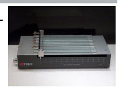
The BK 6 and BK 10 Recorders have independently operating tracks allowing tests to be made at different start times. Pairs of tracks operate at the same speed, and a wide range of travel times are available. Travel times of 6, 12, 24 and 48 hours are all considered as standard. A time scale on the front cover is graduated to suit the instrument's drying time ranges. Each pair of tracks has its own individual operating switch.
