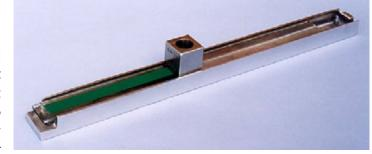
is then positioned on the glass strip at the step end and filled with paint as described above. When using the applicator the casterguide ensures that the film is applied centrally and, as the applicator is drawn off the end of the glass strip, the surplus paint is collected in the trough underneath.
