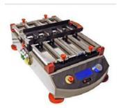
Many standards require dry or wet abrasion and scrub test to be performed to determine the quality of coating. Like the EN 13300 for example. This standard defines a quality ranking for interior coatings to wet abrasion.
