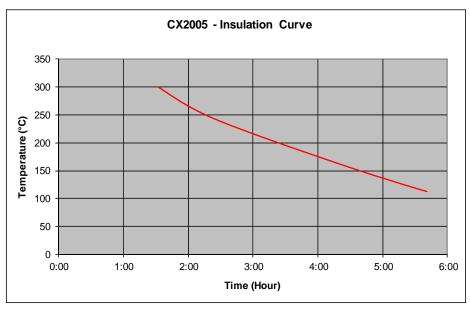
Tested with the **insulation box CX2005** in combination with the **energy absorber CX2011** (a high density energy-collecting media) with a start temperature of 20°C (68°F).
