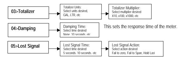
The Lost Signal allows the adjustment of time to hold the last valid flow reading. When this time has elapsed the unit will go to the Lost Signal Action selected.
