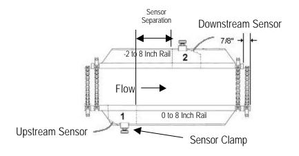
For horizontal pipes, set the longest rail (the one that has a scale of 0 to 8 inches) on top of the pipe and wrap the chains around the pipe and connect the chains to the hook on the thumbscrew assembly.
