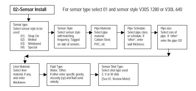
Selecting the Sensor Shot Type will depend on the application. The V-Shot is the easiest to install but the transmitted signal is reflected off the pipe wall and if there is corrosion on the wall this may prevent a good reflected sensor. Switch to the Z-Shot if the meter indicates no signal. The W-Shot is used on 1 or 2 inch pipes.
