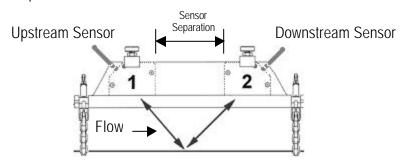
The large sensor mounting rail is used for the V-Shot configuration up to 12 inch pipes. For larger pipes the small mounting rail is used in conjunction with the large rail. The mounting of the rail(s) to the pipe is the same procedure as described in the Z-Shot mounting. It is not necessary for the rail to be level when using the large rail only. But the rail should never be mounted at the top or bottom of a horizontal pipe.
