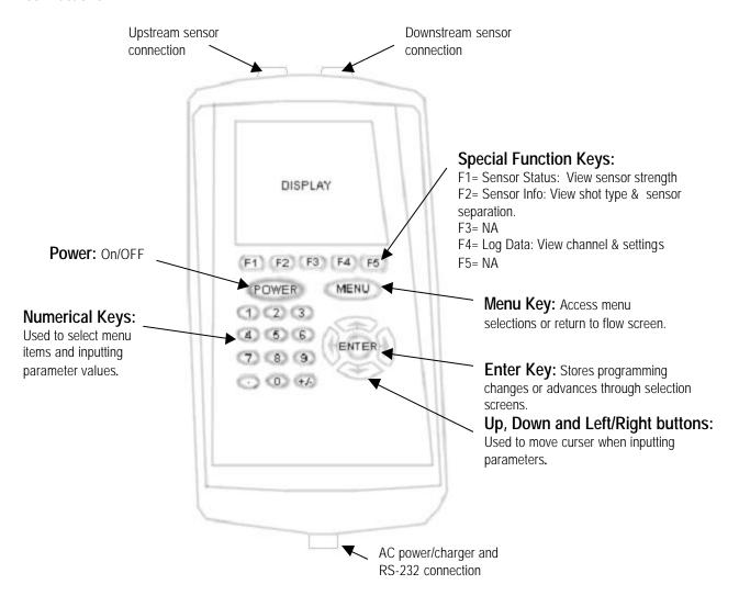
To access the programming sections of the Vantage 6000, press the Menu key. The following list will appear on the display.
