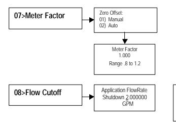
This allows setting or capturing any flow offset in the meter. This is done with zero flow in the pipe. It can be manually set or auto capture.
