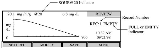
Press the [NEXT REC.] soft-key to change the record number to find an empty slot, or pick a slot to overwrite (you cannot delete results, you must overwright). Press the [SAVE] soft-key to save the current test data into that slot. Once you have saved the data you can press the [MODIFY] soft-key to change the parameters of the test.
