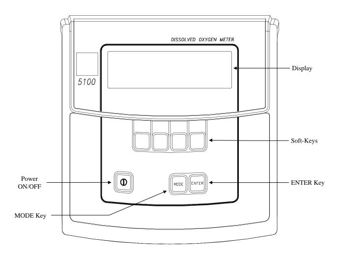
The 5000/5100 has two main operating modes, Main and Application. The current mode is displayed in the dark bar at the top right corner of the display. The following diagram shows the display while the instrument is in the Main mode.
