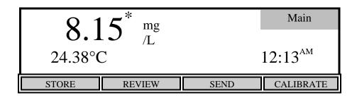
The bottom row of the display shows the functions of the four soft-keys used during Main mode. Main mode is used to make measurements, store or review readings and send the current readings to a computer or serial printer.
