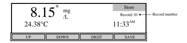
The Store menu is used to control the storing of data. The current record number is shown in the display on the right side.
