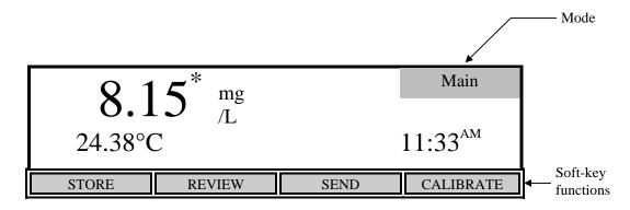
The bottom row of the display identifies the function of the four soft-keys which are located on the keypad below the display. The function of each of these keys changes with each mode.
