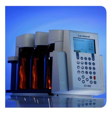
The BD 600 is the ideal system for process control or as a secondary test to the Dilution Method. Using a respirometric system solves many of the issues associated with the dilution method for BOD analysis.
