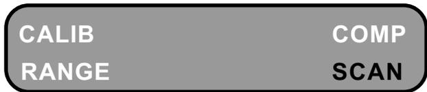
Select the DISPLAY SCAN RATE for the Mark 24. The default is SLOW and is indicated by flashing SLOW in the display. Use the UP ARROW or DOWN ARROW key to select a different SCAN RATE. The scan rates for SLOW (8 sec.), MEDIUM (4 sec.) and FAST (2 sec.) are preprogrammed and cannot be changed. Now Depress the ENTER key to use this selection.
