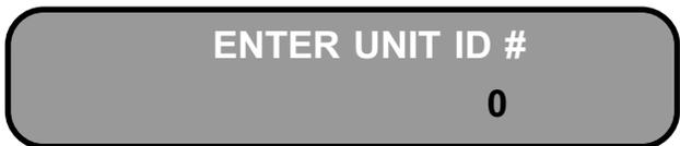
The Mark 24 will then momentarily display the UNIT ID ENTERED. After displaying the UNIT ID ENTERED prompt, the Mark 24 exits the SET ID/PW function and displays the SETUP MAIN MENU.
