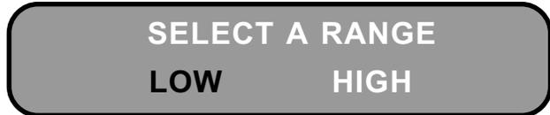
The Mark 24 then displays the SETUP MAIN MENU. The set RANGE function can then be exited from the main menu.
