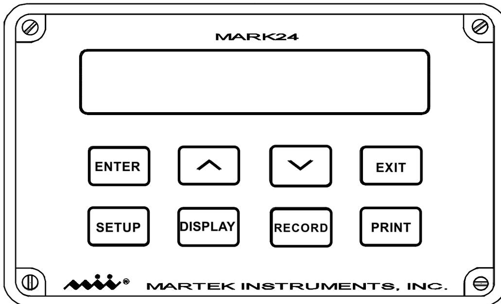
Figure 3.1 - Mark 24 Front Panel
