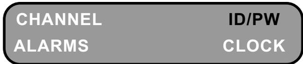
Select the ID/PW function you wish to perform. The default selection is PASSWORD and is indicated by the flashing PASSWORD prompt. Use the UP ARROW or DOWN ARROW key to select the ID # function. When selected the ID/PW prompt flashes. Now depress the ENTER key to use this selection.
