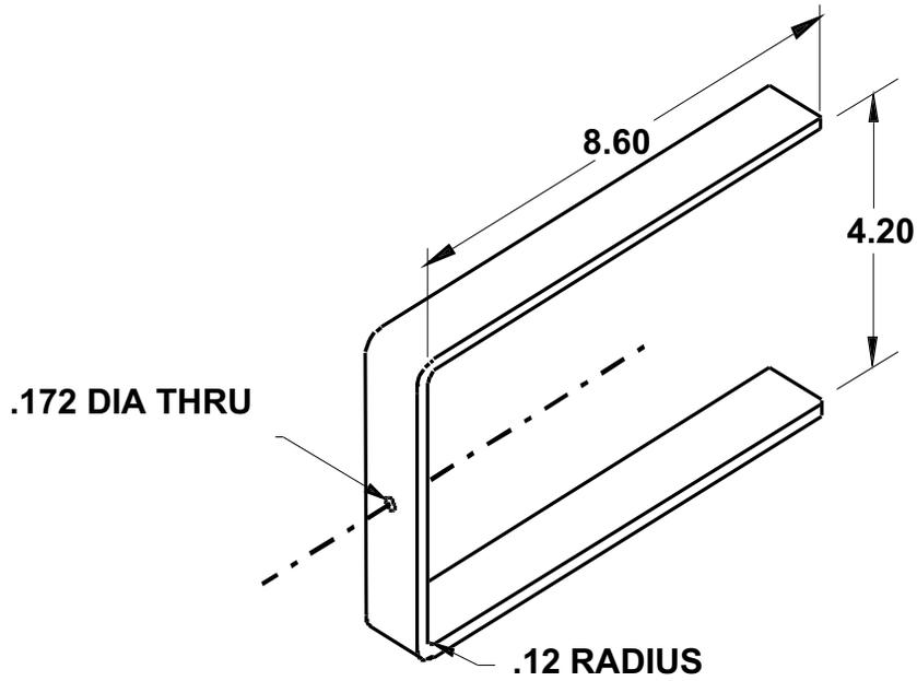
Fig 2.2 Mark 24 Panel Mounting Bracket (P/N 820930)
