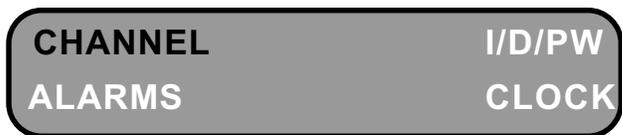
Select the SETUP function you wish to perform. Use the UP ARROW or DOWN ARROW key to select the SCAN function. When selected, the SCAN prompt flashes. Now depress the ENTER key to use this selection.
