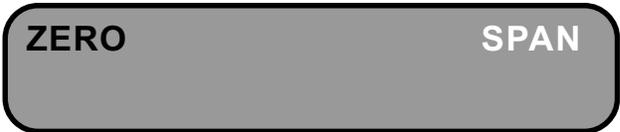
This prompt is displayed for a short time. This allows the user to place the TEMP - RUN jumper in the preamp in the 0° C position for electronic calibration or place the temperature sensor in a low temperature solution standard.
