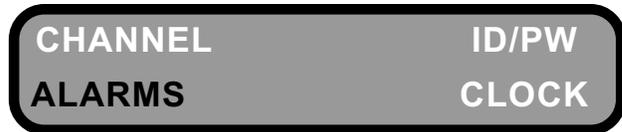
This is the **ALARM MENU**. Select the **ALARM** function you wish to perform. The default selection is **ALM MODE** and is indicated by the flashing **ALM MODE** prompt. Use the **UP ARROW** or **DOWN ARROW** key to select the desired function. Now depress the **ENTER** key to use this selection.
