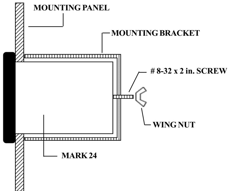
Fig 2.3 Mark 24 Panel Mounting - Side View
