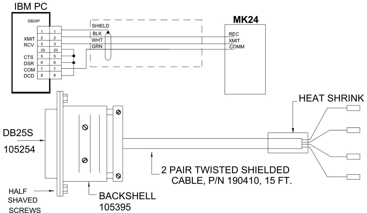
Fig. 2.12 RS232 CABLE ASSEMBLY
