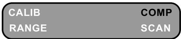
Select the type of channel you wish to compensate. The default channel type is COND, indicated by the flashing COND in the display. Use the UP ARROW or DOWN ARROW to select either pH or COND type of channel. Now depress the ENTER key to use this selection.
