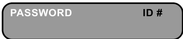
The screen allows the user to enter a SINGLE DIGIT unit identification number. The current unit ID # appears in the second line of the display. This digit will be flashing indicating that this digit may be changed to any number between 0 - 9. This number may be incremented using the UP ARROW key or decremented using the DOWN ARROW key. When the ID number equals the desired value depress the ENTER key to save the value.
