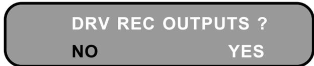
The Mark 24 displays the **drive ONE** or **ALL RECORDER CHANNELS** selection menu. Use the **UP ARROW** or **DOWN ARROW** key to select the desired function. For this example select **ONE CHN**. Depress the **ENTER** key to use this selection.
