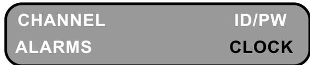
This is the **CLOCK MENU**. Select the **CLOCK** function you wish to perform. The default selection is **DATE** and is indicated by the flashing **DATE** prompt. Use the **UP ARROW** or **DOWN ARROW** key to select the desired function. Now depress the **ENTER** key to use this selection.
