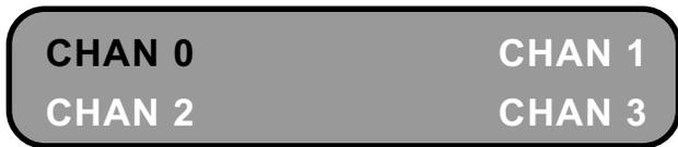
The Mark 24 displays **CHANNEL RECORD MODE** for the selected channel on the first line of the display and the **RECORDER RANGE** on the second line of the display. The display format for the range is defined in the **SET RECORD RANGE** function. This display screen is displayed for 6 seconds **ONLY**.
