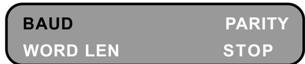
*The Mark 24 displays the list of available baud rates supported by the Analyzer. Use the UP ARROW or the DOWN ARROW keys to select the desired BAUD RATE you wish to set for the serial port. The default selection is 9600. Select 9600 and depress the ENTER key to save this selection.*
