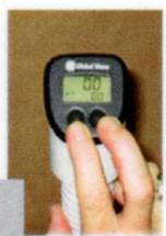
Reset the display computer by pushing both Right & Left buttons simultaneously. Scroll to "V" Mode to measure velocity (to nearest 0.1 ft/sec; Avg & Max to nearest 0.01 ft/sec).
