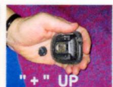
Replace the battery with the " + " side up.
