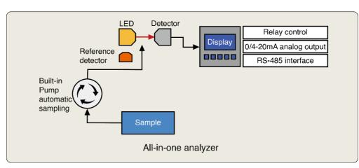
Incident light from the LED is measured at an angle of 180 degree. The detector receives the signal formed by the amplified converter and signal conversion to digitally displayed. in addition to the signal detector, there is a reference detector at the side of the LED light source. It offers an automatic compensation system, and prevents distortion of signal by the deterioration of sensor LED.
