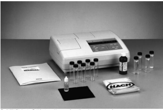
The 2100N IS Laboratory Turbidimeter combines ease-of-use with consistent, accurate performance.
