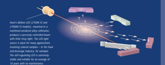
With a back-scatter detector, 2100AN and 2100AN IS models are uniquely equipped to measure high levels of turbidity (up to 10,000 NTU) with excellent accuracy.
