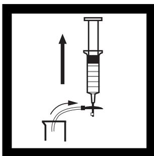
**2.** Fill a beaker or container with the water to be filtered. Insert the tubing into the container. Slowly draw about 50 mL water into the syringe by pulling up on the syringe plunger.
