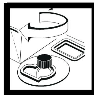
4. Lift the cell compartment cover, rotate the sample cell (approximately 1/8 of a turn). Close the lid, press **ENTER** and record the reading. Continue this procedure until the smallest FNU reading is obtained.
