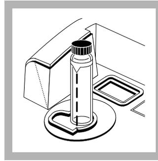
**3.** Select the StablCal vial labeled < 0.1 NTU. Wipe the cell clean and apply a thin film of silicone oil to its surface. Place it in the cell holder and close the cell cover. Press **ENTER**.
