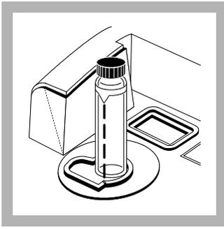
**5.** Select the StablCal vial labeled 200.0 NTU. Wipe the vial clean and apply a thin film of silicone oil to its surface. Place it in the cell holder and close the cell cover. Press **ENTER**.
