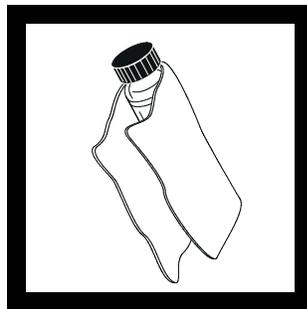
**3.** Wipe the sample cell clean, and apply a film of silicone oil (refer to Section 2.3.2).
