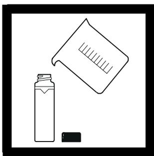
1. Fill the clean cell to the line with high-quality water, and cap the sample cell (refer to Section 2.3.3).
