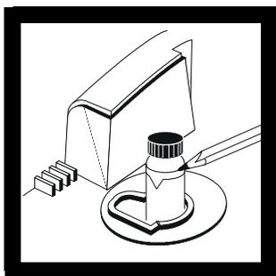
5. Place an orientation mark on the sample cell marking band adjacent to the index mark. Use this mark to align the sample cell each time a measurement is made.
