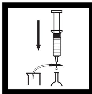
**3.** Slowly push on the plunger to force the water through the filter and into a graduated cylinder or volumetric flask. Repeat Steps 2 and 3 until the desired amount of water is obtained.
