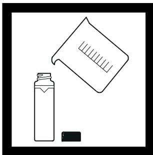
**10.** Fill a clean sample cell to the line with well-mixed, 1000-FNU formazin standard. Wipe the cell clean and apply a thin film of silicone oil to the surface. Place it in the cell holder and *close the cell cover*. Press **ENTER**. The instrument display counts down from 60 to 0, and then takes a measurement.
