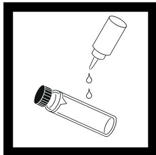
**2.** Apply a thin bead of silicone oil from the top to bottom of the cell—just enough to coat the cell with a thin layer of oil.
