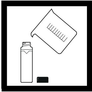
**1.** Collect a representative sample in a clean container. Fill the sample cell to the line (approximately 30 mL). Take care to handle the sample cell by the top. Cap the sample cell.
