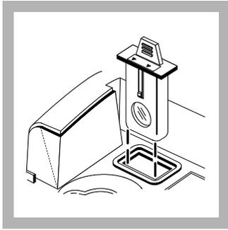
**1.** Insert the EPA filter module if measuring for EPA-reporting (2100N and 2100AN only).
