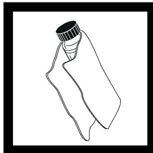
**3.** Spread the oil uniformly using the oiling cloth provided. Wipe off the excess leaving only a thin coat. The cell should appear nearly dry with little or no visible oil.
