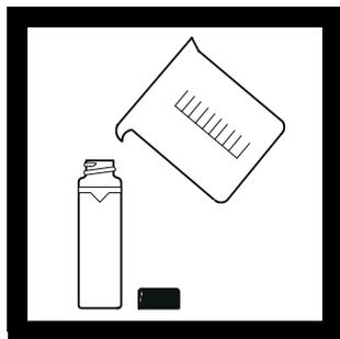
**9.** Fill a clean sample cell to the line with well-mixed, 200-FNU formazin standard. Wipe the cell clean and apply a thin film of silicone oil to the surface. Place it into the cell holder, and *close the cell cover*. Press **ENTER**. The instrument display counts down from 60 to 0, and then makes a measurement. The instrument automatically increments to the next standard, the display shows 1000 FNU, and the S3 annunciator flashes. Remove the sample cell from the instrument.
