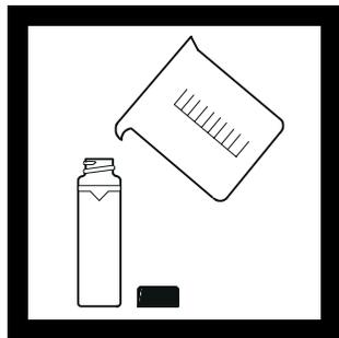
**2.** Fill a clean sample cell to the line (approx. 30 mL) with dilution water.
