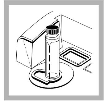
**4.** Select the StablCal vial labeled 20.00 NTU. Wipe the vial clean and apply a thin film of silicone oil to its surface. Place it in the cell holder and close the cell cover. Press **ENTER**.
