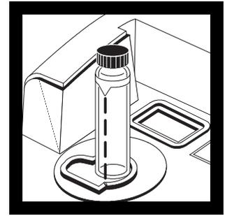
**4.** Place the sample cell in the instrument cell compartment and close the lid.
