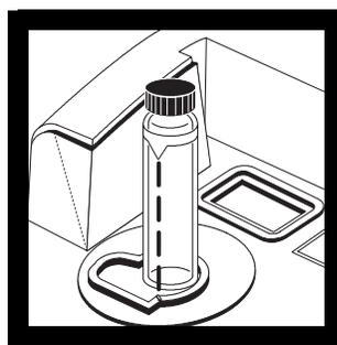
3. Insert the sample cell into the cell compartment, and close the cell cover. Record the reading.
