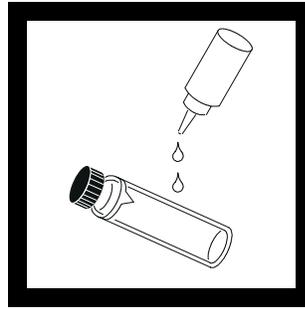
**3.** Apply a thin bead of silicone oil from the top to bottom of the cell—just enough to coat the cell with a thin layer of oil. Using the oiling cloth provided, spread the oil uniformly. Then, wipe off the excess. The cell should appear nearly dry with little or no visible oil. See Section 2.3.2.
