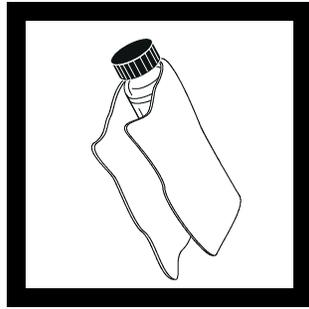
**2.** Hold the sample cell by the cap, and wipe to remove water spots and finger prints.
