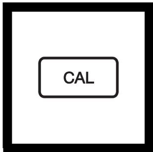
**1.** Press **CAL**. The CAL mode annunciator lights, and the S0 annunciator flashes. The FNU value of the dilution water used in the previous calibration is displayed.
