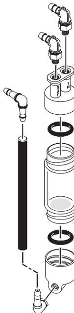
Sample is introduced into the top of the cell. A baffle deflects the incoming sample to the side wall of the cell, minimizing turbulence in the light path.
