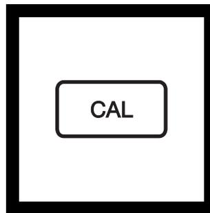
**11.** Press **CAL**. The instrument makes calculations based on the new calibration data, stores the new calibration and returns the instrument to the measurement mode.
