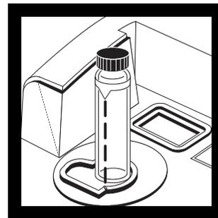
**4.** Place the capped sample cell into the cell holder, and close the cell cover.
