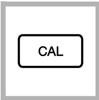
**9.** Press **CAL/Zero**. The instrument makes calculations based on the new calibration data, stores the new calibration and returns to measurement mode.
