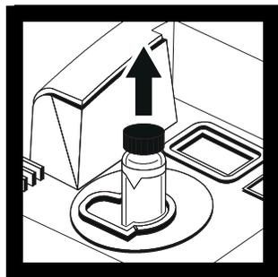
**6.** The instrument automatically increments to the next standard, displays the expected FNU value (e.g., 20.00 FNU), and the S1 annunciator flashes. Remove the sample cell from the cell holder.
