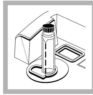
**7.** Select the StablCal vial labeled 4000 NTU. Wipe the vial clean and apply a thin film of silicone oil to its surface. Place it in the cell holder and close the cell cover. Press **ENTER**.
