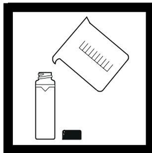
**7.** Fill a clean sample cell to the line with well-mixed, 20-FNU formazin standard. Wipe the sample cell clean, and apply a thin film of silicone oil on its surface. Place it into the cell holder, and close the cell cover.
