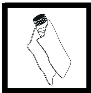
2. Wipe the sample cell clean, and apply a film of silicone oil (refer to Section 2.3.2).
