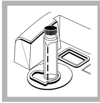
**6.** Select the StablCal vial labeled 1000 NTU. Wipe the vial clean and apply a thin film of silicone oil to its surface. Place it in the cell holder and close the cell cover. Press **ENTER**.
