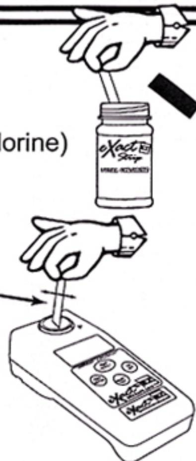
\*NOTE: Standard Method (4500-Cl G, simplified procedure for total chlorine) requires the reading to be made after a 2 minute wait. From experience, water samples above 68°F, generally, do not require the full 2 minute wait.
