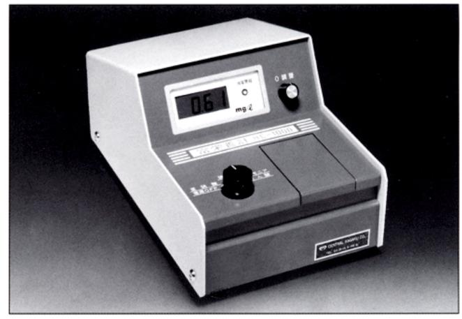
An in crease in nutritious substances in water gives rise to abnormal growth of water-bloom or red tide. This in turn gives rise to harmful effects, for example, giving foul smell to drinking water and causing death to fish. This is a portable photoelectric instrument allowing quick and easy quantification of the phosphorus and nitrogen content of the water. Both sustances are factors that regulate the growth of plant plankton.
