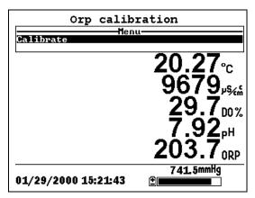
Figure 6.16 ORP Calibration Screen
