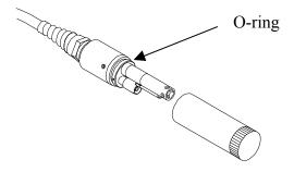
Figure 3.7 Transport/Calibration Cup Installation
