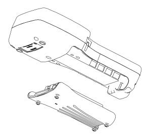
Figure 2.4 Inserting Battery Pack
