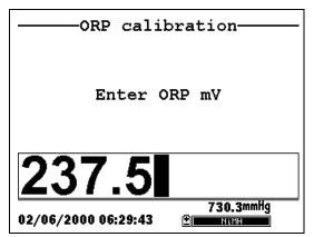
Figure 6.15 Specified ORP Calibration Screen
