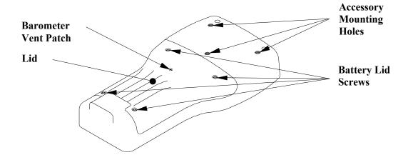
Figure 2.2 Back View of YSI 556 MPS
