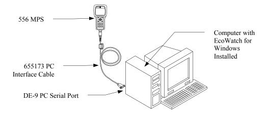
Figure 8.6 Computer/Instrument Interface
