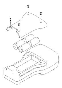
Figure 2.3 Inserting C Cells
