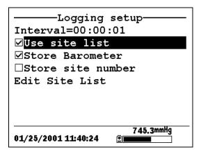
Figure 9.6 Logging Setup Screen
