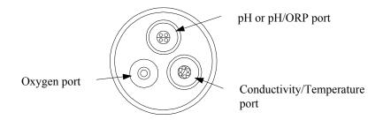
Figure 3.3 Sensor Port Identification
