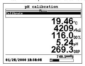
Figure 6.14 pH Calibration Screen
