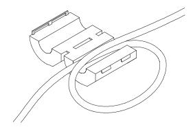
Figure 19.1 Ferrite Bead Installation
