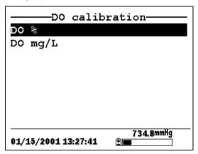
Figure 6.7 DO Calibration Screen
