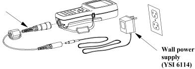
Figure 2.5 Charging the Battery Pack
