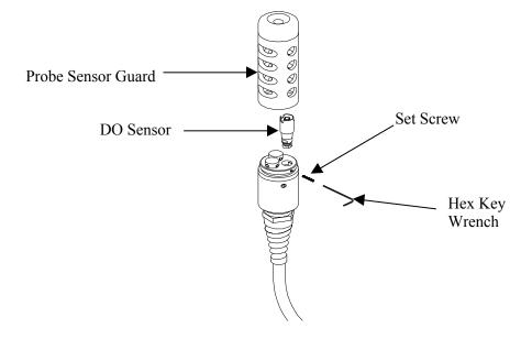
Figure 11.1 DO Sensor Replacement
